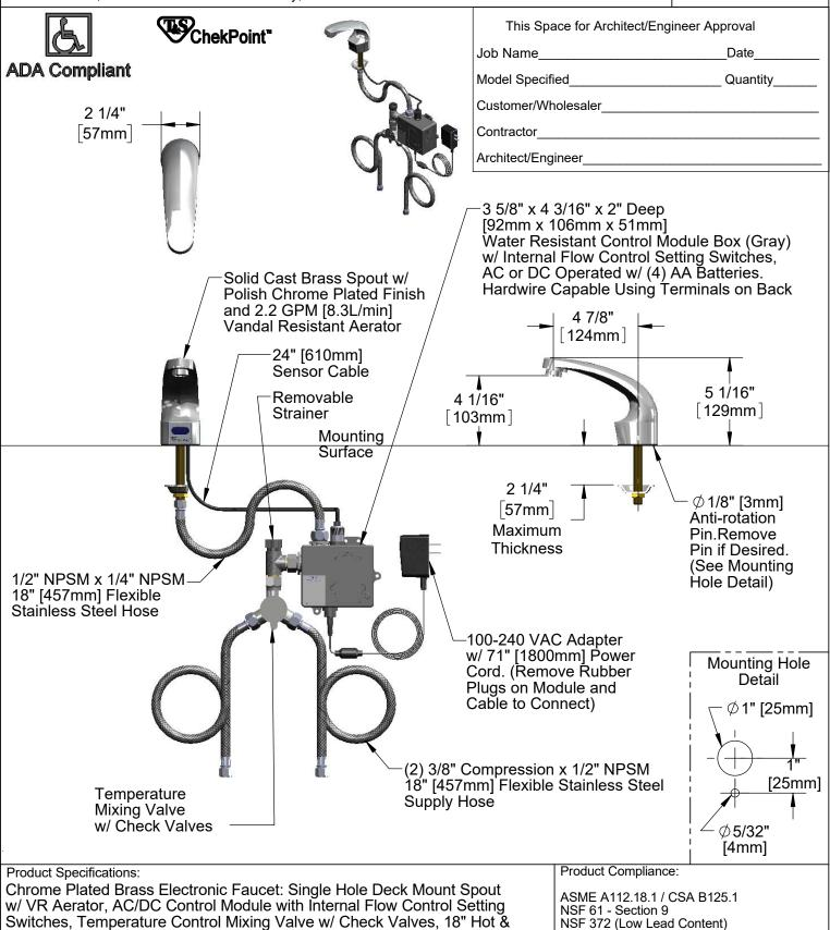
Switches, Temperature Control Mixing Valve w/ Check Valves, 18" Hot &
