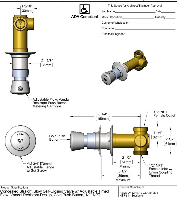
Female Outlet and 1/2" NPT Female Inlet w/ Union Coupling
