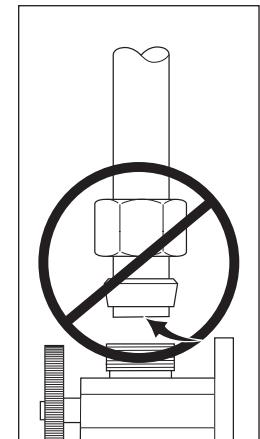
**Ensure tube is fully inserted into stop before sliding sleeve down to engage top of fitting.**
